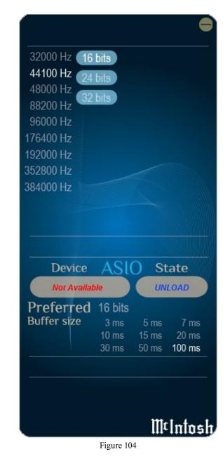
3. When the Media Stream Program on the computer is set to output in the "ASIO" format, the McIntosh -HD USB Audio Control Panel allows for changing the settings parameters on the fly.
