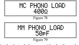
3. Set the desired phono cartridge loading value (Ohms for a Moving Coil Cartridge or Capacitance for a Moving Magnet Cartridge) that comes closest to the Phono Cartridge Makers recommended value. After approximately 6 seconds the Alphanumeric Display returns to indicate the Source Selection and Volume Level.
