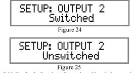
The C52 Default Setting for using Headphones is to automatically mute all the Output Connectors when the Headphone Cable Plug is inserted into the C52 Front Panel HEADPHONES Jack. There are three available settings:
