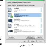
to the computer, an additional "McIntosh USB Audio" playback device will appear in the listing. Make sure to select the "McIntosh-HD HS USB Audio" from available plavback devices listed when using this McIntosh Product for USB Audio.
